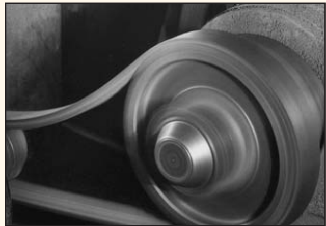
A Ramsey Silent Chain operating at high speed. Note the smoothness and lack of vibration
