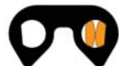
SC chain joint with "D" shaped pins
