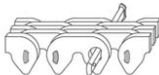
Insert longer pin through the chain.
