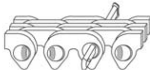
Insert longer pin through the chain.
